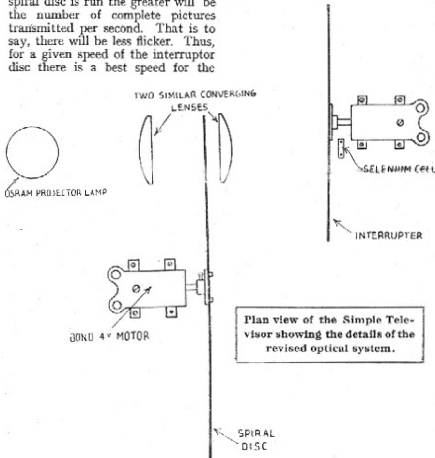
Plan view of the Simple Televisor showing the details of the revised optical system.
